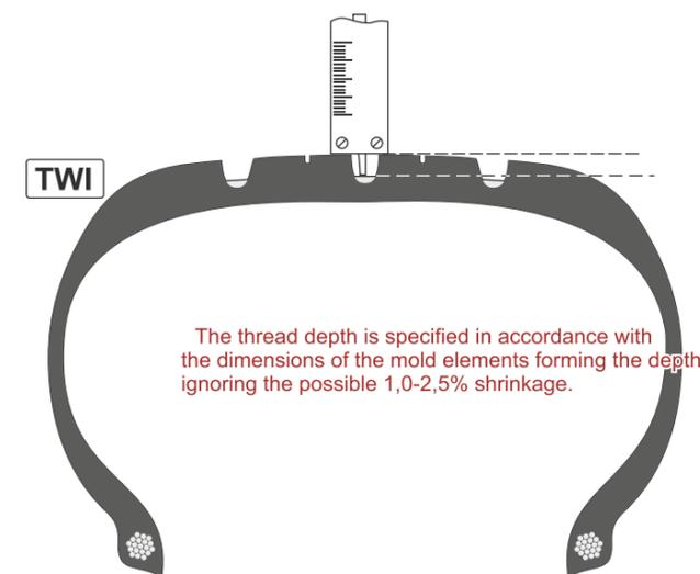
The thread depth is specified in accordance with the dimensions of the mold elements forming the depth ignoring the possible 1,0-2,5% shrinkage.
